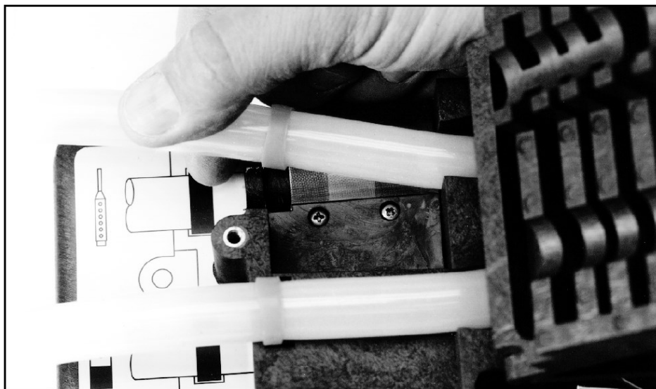
Figure 21 - Removing and replacing the pump tube, from ISCO AVALANCHE user manual, page 9-10.
