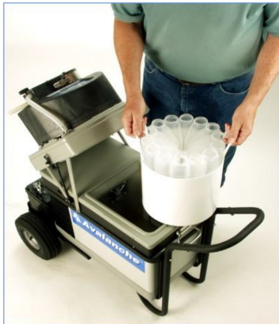
Figure 16 - Bottle Carrier with 14 Bottles 950ml.
