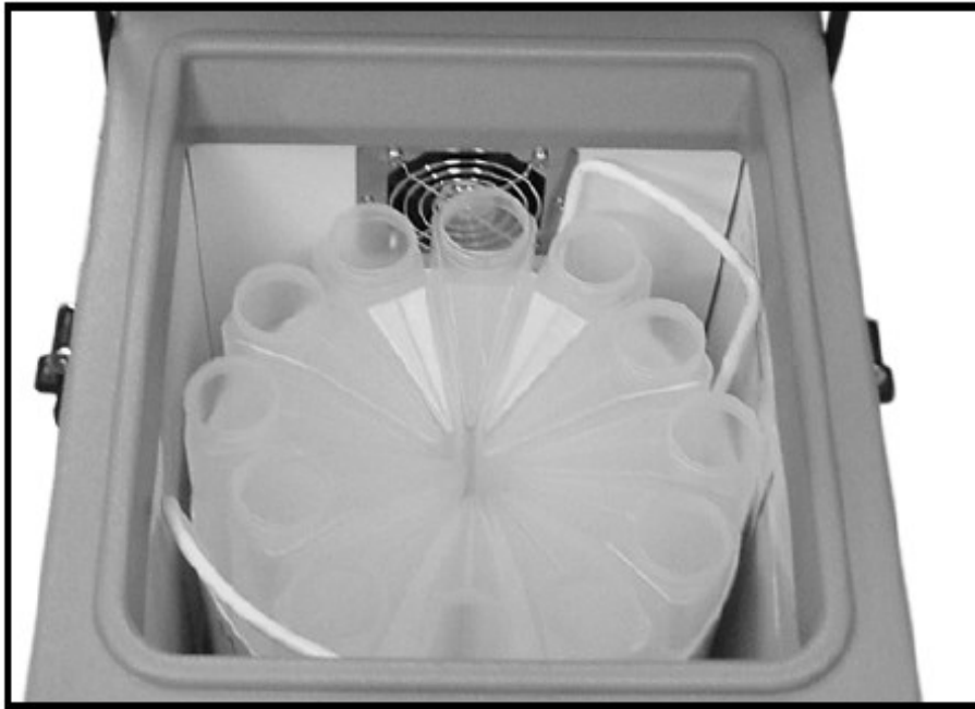
Figure 24 - 14-Bottle configuration completed, from ISCO AVALANCHE user manual, page 2-7.
